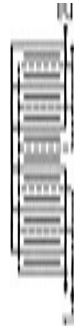
2 pass-2 plate exchanger with overall parallelflow and individual passes in parallelflow, stream symmetric
